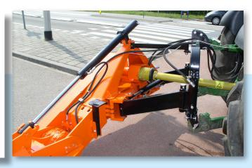
A unique large deflection breakaway device ensures maximum protection. The pto power is transmitted to the flail rotor through a 5-fold power belt, which is automatically kept at the right tension. A flexible coupler eliminates peak strokes on the drive system.
