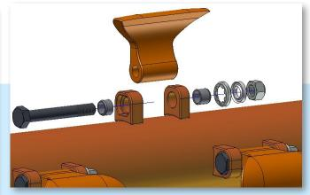
The standard 2,2 kg (5 lbs) special flails are fitted to the large diameter double balanced rotor with with heavy 20 mm bolts and replaceable steel bushes.PERFECT Combi-flails are optional avialbale.
