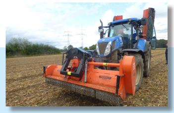
The mid mower can be mounted in the tractor 3-pt. linkage with a special "pulled type" headstock. Or behind the two mid mowers at the special frame.
