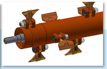
The 0,9 kg (2 lbs) special flails with single cutting edges ensure clean and finest cut of grass, rushes, reed stems, pruning etc. up to 3 cm. They are fitted to the double balanced rotor with with heavy 20 mm bolts and replaceable steel bushes.
