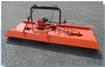
The indirect, flexible V-belt drive of all rotor spindles protects the gearbox and the PTO shaft against shockloads. V-belt tension is easily adjustable. Mostbelts have an automatic spring loaded belt tensioner.
