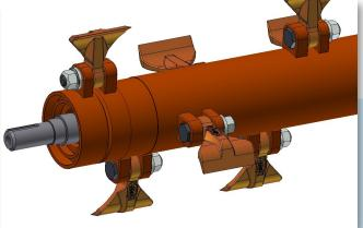
The 0,9 kg (2 lbs) special flails with single cutting edges ensure clean and finest cut of grass, rushes, reed stems, pruning etc. up to 3 cm. They are fitted to the large diameter double balanced rotor with with heavy 20 mm bolts and replaceable steel bushes. 2,2 kg universal flails, or Combiflails are optional avialbale.
