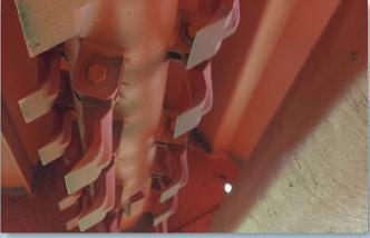
Special PERFECT 0,9 kg flails with a straight, continuous cutting edge guarantee an excellent cut, uniform cutting height and even spread of the grass over the rear roller.
